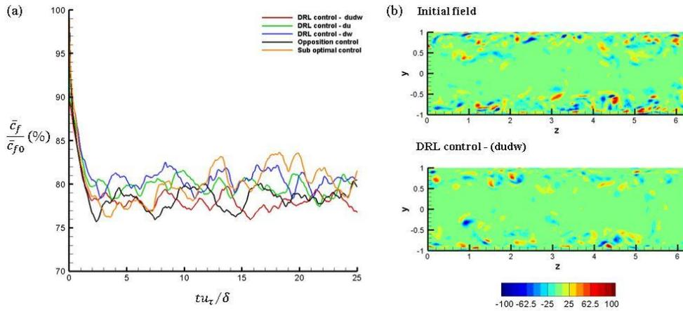
Figure 1 (a) Drag reduction plot and (b) Vorticity contour
